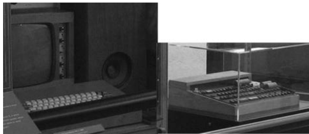
FIGURE 7.12 Apple I built in a wooden box. (Courtesy of Alpha1, http://commons.wikimedia.org/wiki/File:Apple_1_computer.jpg .)
