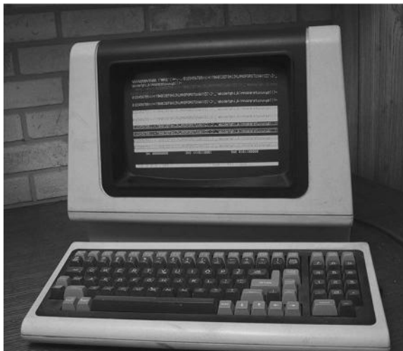
FIGURE 7.11 A dumb terminal, circa 1980. (Adapted from Wtshymanski, http://en.wikipedia.org/wiki/File:Televideo925Terminal.jpg .)
