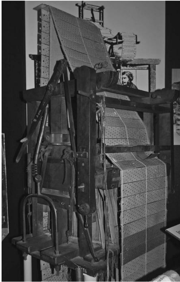
FIGURE 7.4 Jacquard's programmable loom. (Mahlum, photograph from the Norwegian Technology Museum, Oslo, 2008, http://commons.wikimedia.org/wiki/File:Jacquard_loom.jpg .)
