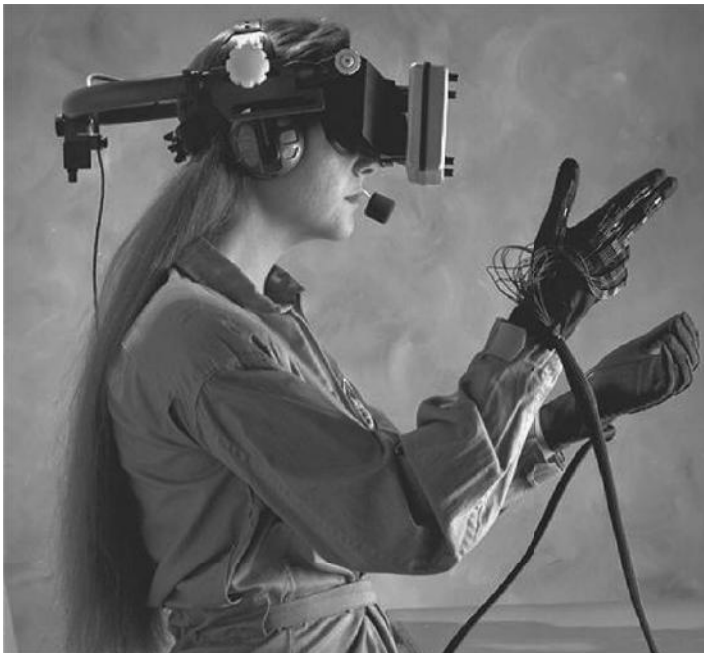
FIGURE 2.8 Virtual reality headset and data glove in use. (Courtesy of NASA, http://gimp-savvy.com/cgi-bin/img.cgi?ailsxmzVhD8OjEo694 .)
